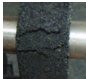
non-modified asphalt shingle with cracking
