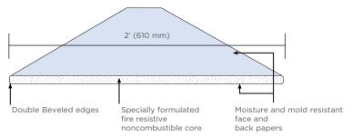
GlasRoc\* and M2Tech\* Shaftliner are designed and engineered for use in construction of lightweight Shaftwall and Area Separation Firewalls. These systems are UL, cUL, and ULC listed for fire resistance. GlasRoc\* and M2Tech\* Shaftliner can be substituted with each other.
