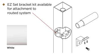
Note: Handrail depicted is not free standing and must be anchored to walls or guardrail using handrail bracket assembly (74028/74029). Space a maximum of 6' on center and as close as possible to both sides of any joint. (ADA compliant at 6ft spans)
