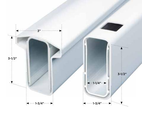
For safe, secure vinyl railing applications, there's no better choice than the Oxford routed system. The routed Oxford system features a unique internal rail-to-post connection and hidden hardware, so there are no unsightly brackets to detract from the look of the railing. The aluminum reinforced rail connects to a sturdy galvanized post support kit inside the routed post, for a completely concealed metal-to-metal connection.
