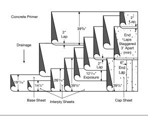
\* For systems substituting ply sheet for the base ply, install all ply sheets in a shingled pattern. Exposure and starter dimensions should be adjusted accordingly to obtain required coverage and headlap, per NRCA recommendations.
