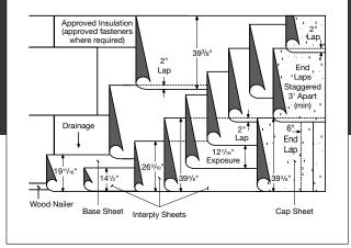
Premium Alternate. Over a base sheet or bonded to a primed substrate. One smooth modified membrane and CT SmartFlash<sup>®</sup>, per CT detail.
