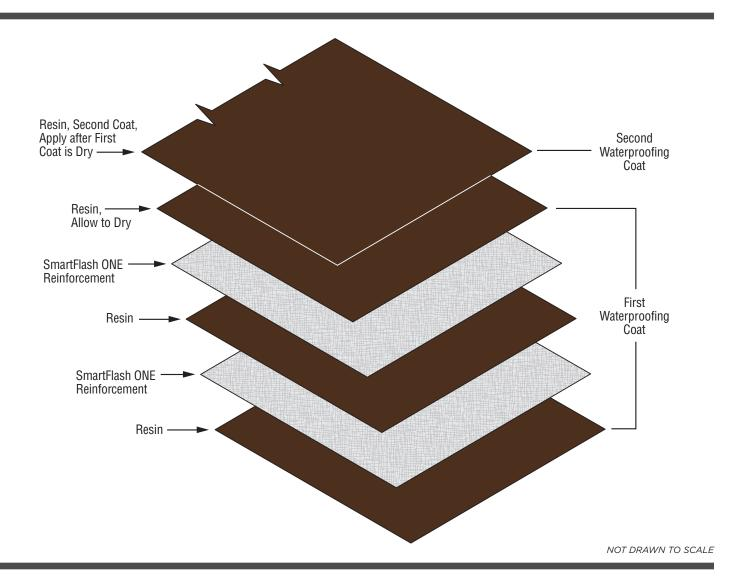
NOTE: The first waterproofing coat will not be dry enough for foot traffic after 2-3 hours; the second waterproofing coat shall be able to be applied without standing on the flashing area.
