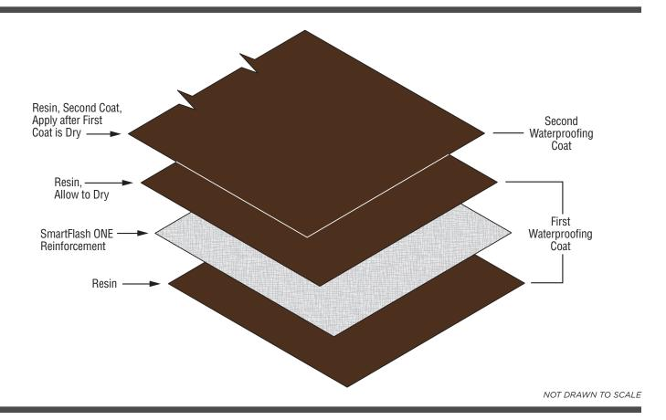
NOTE: The first waterproofing coat will not be dry enough for foot traffic after 2-3 hours; the second waterproofing coat shall be able to be applied without standing on the flashing area.
