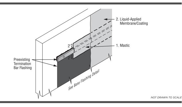
NOTE: Never repair or coat-over silicone-based mastic or coating with anything other than a compatible silicone-based product; acrylic materials will not bond to silicone.
