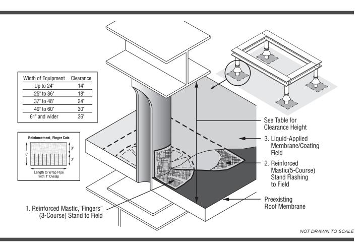
NOTE: Never repair or coat-over silicone-based mastic or coating with anything other than a compatible silicone-base product; acrylic materials will not bond to silicone.
