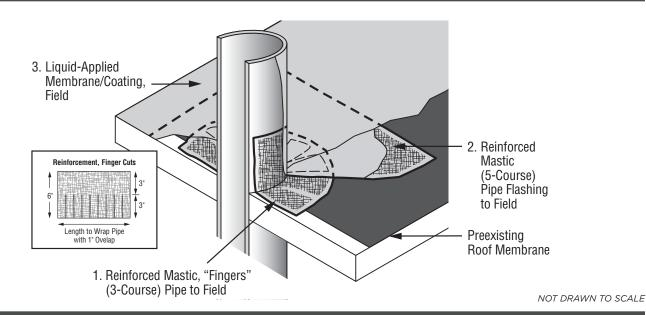
NOTE: Never repair or coat-over silicone-based mastic or coating with anything other than a compatible silicone-based product; acrylic materials will not bond to silicone.
