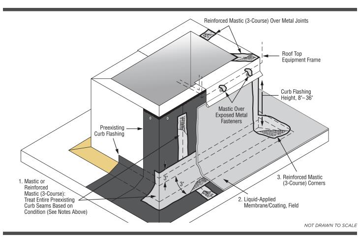
NOTE: Never repair or coat-over silicone-based mastic or coating with anything other than a compatible silicone-based product; acrylic materials will not bond to silicone.
