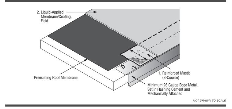
NOTE: Never repair or coat-over silicone-based mastic or coating with anything other than a compatible silicone-based product; acrylic materials will not bond to silicone. If new metal is installed, clean and remove any oil or residue that could inhibit adhesion.
