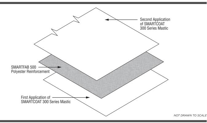
NOTE: SMARTCOAT 300 Acrylic Mastic and SMARTCOAT 350 Silicone Mastic are recommended when 3-coursing is required; SMARTCOAT 301 and SMARTCOAT 365 Mastics are fiber reinforced; saturating through polyester can be challenging.
