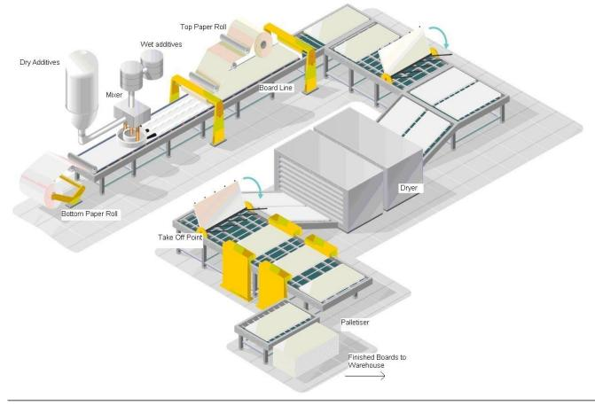
Gypsum, the main raw material, comes from one of four sources: FGD is transported from power stations, natural gypsum is extracted from mines and quarries, process scrap is reformed into new product and construction/demolition waste is collected from jobsites and returned to the plant for reprocessing. This material is calcined before use to produce the hemihydrate of calcium sulphate — stucco (CaSO4•½ H2O). This stucco is stored in silos.
