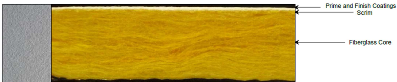
Figure2: Diagram of Symphony f Ceiling Panel Construction
