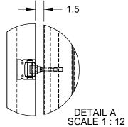
Gate hinge threads into the upper and lower inserts in the gate metal frame leaving about 1.5" from the edge of the gate to the post.
