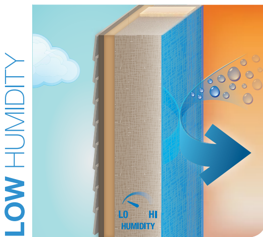
Remains moisture tight in winter when humidity in the cavity is low.
