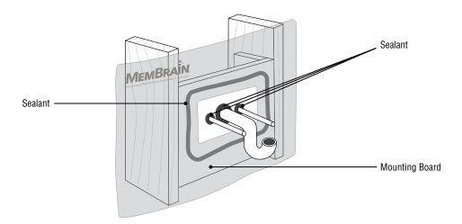
Figure 14: Mounted and sealed plumbing penetrations.
