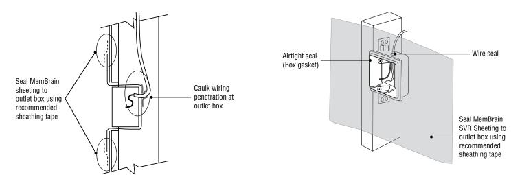
Figure 12: Sealed interior electrical outlet.
