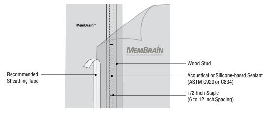
Figure 5: Overlapping seam treatment.
