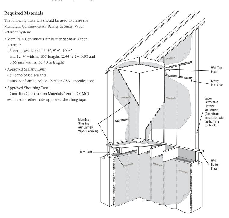
Figure 1: Maintain air barrier continuity at rim joists, corners, partition wall interfaces and ceilings.
