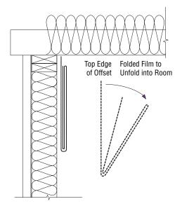
Figure 2: MemBrain sheeting orientation for wall installation method.
