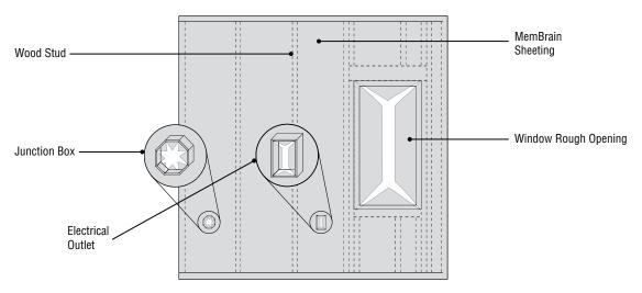
Figure 7: Cut MemBrain sheeting to tightly fit penetrations.
