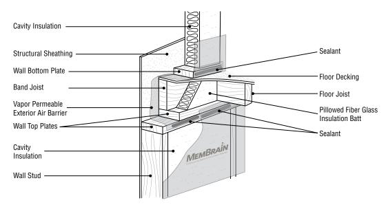
Figure 17: Detail B – MemBrain Air Barrier System interior floor intersection details.
