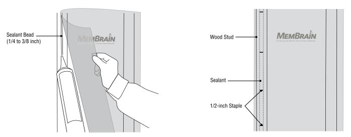
Figure 3: Sealant application.
