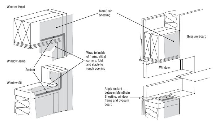
Figure 8: Window rough-opening treatment.
