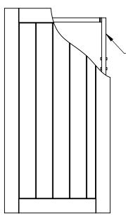
Gate is reinforced with a 1.5" galvanized steel box tube
