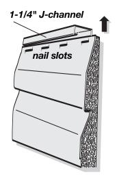
When you cut a siding panel to fit around an opening, use a nail slot punch to create additional nail slots. Fasten through these additional nail slots to secure the panel. Make sure the face of the J-channel or other trim will cover the nail slots.
